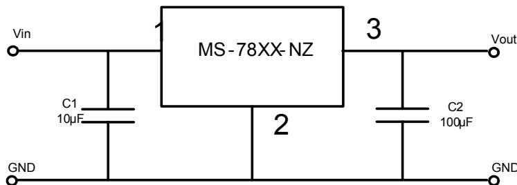
**C1:** A low ESR capacitor is required to keep the noise of the converter to a minimum.
